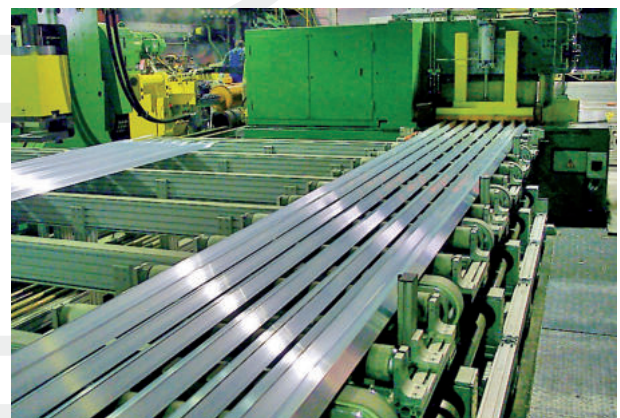
Layer saw for aluminium tubes and profiles, arranged in the runout of an extrusion press 置于挤压机出料部位，用于铝管材、铝型材的层锯
