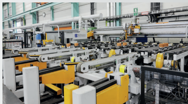
Sawing unit with special feed system for copper tubes and bars
