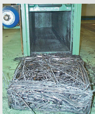
Discharge chute of swarf press, with swarf pressed in to a package
