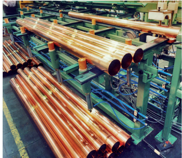
Tube expanding device for swarfless cut copper tubes 用于铜管无屑切割的管材扩张装置
