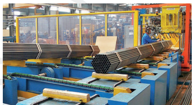
Bundle transport and draining station for steel tubes 钢管成捆运输装置和排放站
