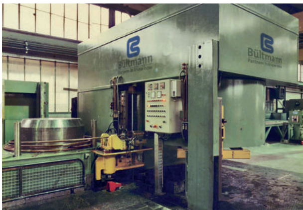
Bull block with hanging drum for copper and copper-alloyed tubes 铜及铜合金管材盘拉机，配备悬挂式转筒
