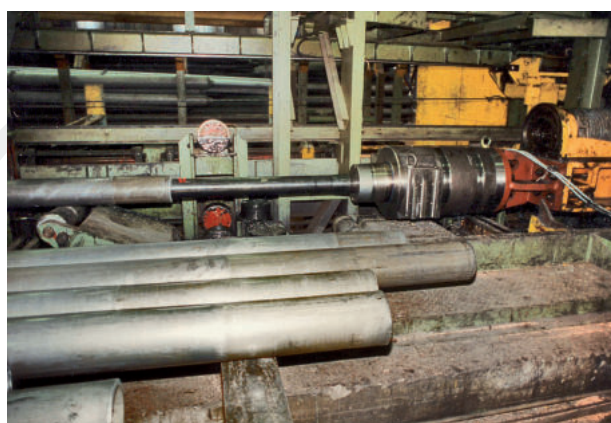
Single internal gripper system for large steel tubes, designed for a drawing force of 3000 kN 拉力达3000千牛的大尺寸钢管配套的单一内部夹持系统
