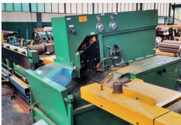
Layer saw for brass tubes and profiles, working in line with drawing and straightening equipment
