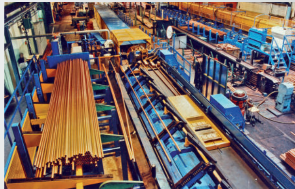
Tube production line for copper tubes with automatic tube separation, pointing machine, triple drawing machine and sawing equipment
