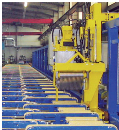
Puller within the runout of an extrusion press for aluminium tubes and profiles 置于铝管材铝型材挤压机出料部位内的拉出装置
