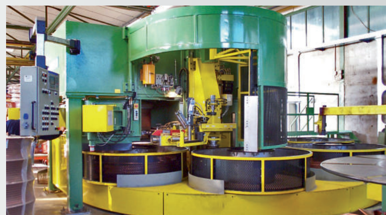
Spinner block for copper tubes, installed at ground level 安装于地表的铜管盘拉机
