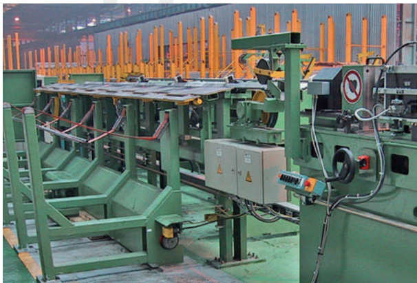
Testing line with Eddy current testing, arranged behind visual testing of steel tubes 置于钢管外观检测后方的涡流探伤生产线
