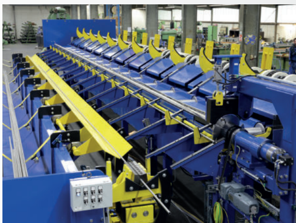
Automatic tube separation, installed upstream of a pointing machine for steel tubes 钢管轧尖机前部的自动管材分放设备
