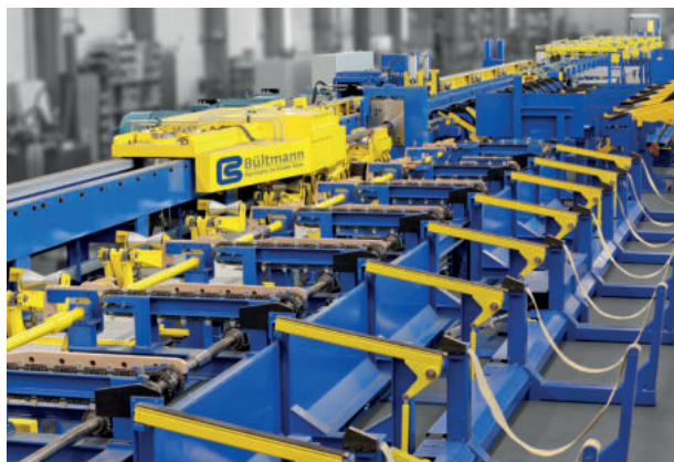
Single tube drawing line for precision steel tubes, with changing device for mandrel rods
