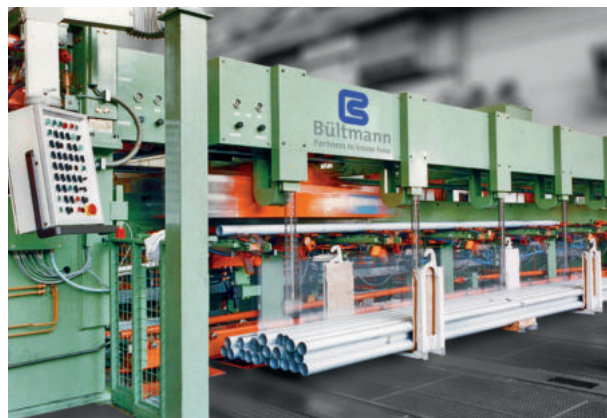
Double tube drawing line for aluminium tubes, with vacuum handling
