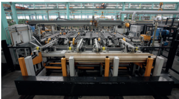
Special stacking system for delicate brass tubes and bars 为精密铜管材铜棒材设计的特殊堆垛系统
