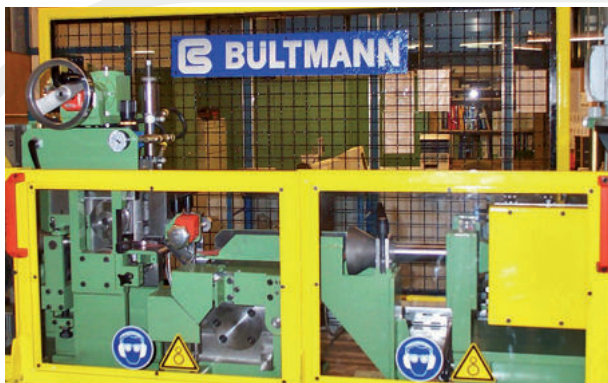
Scrap chopper for plastic coating and copper tubes 用于塑料涂层和铜管的废料碾磨机
