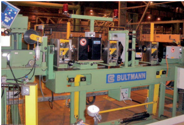
Testing table with Eddy current testing for steel tubes 钢管涡流探伤的测试台
