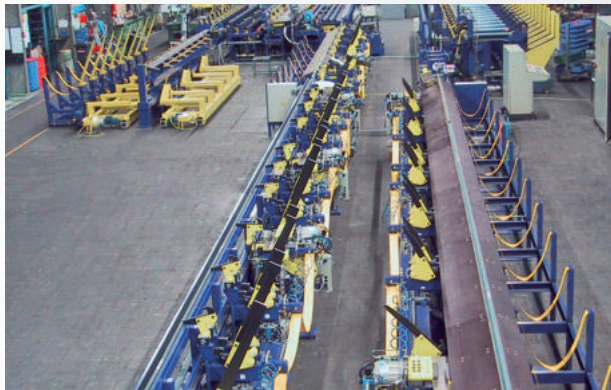
Tube production line for special steel tubes with automatic tube separation, testing unit, sawing equipment, capping device and tube discharge system
