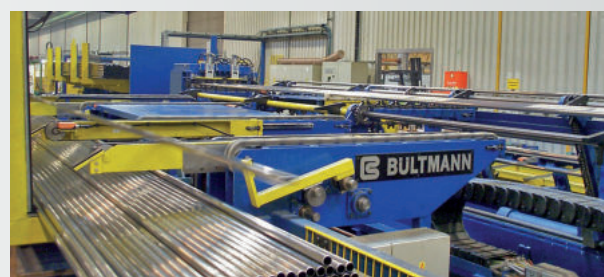
Swarf blow-off unit for steel tubes, with chamfering machine
