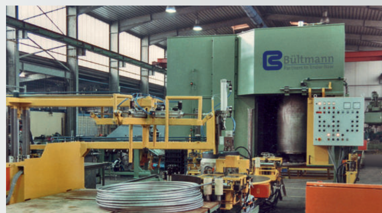
Bull block with vertical drum for steel tubes, push-point- ter and device for feeding the point into the die 用于钢管的盘拉机·配有垂直卷筒、推动型压尖机以及推 动尖端入模具的装置
