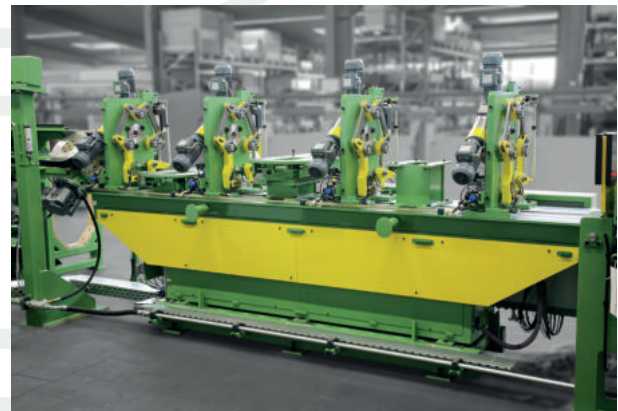
Testing table with precision triple pinch roll units and with sliding tables for testing electronics 配有精密三重夹送辊装置的检测台以及检测电子器件的滑动测试台
