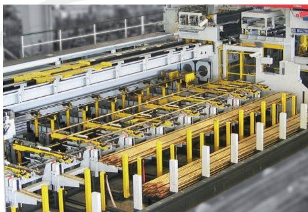
Double tube drawing line for copper and copper-all-oyed tubes, driven by toothed rack, with automatic tube separation
