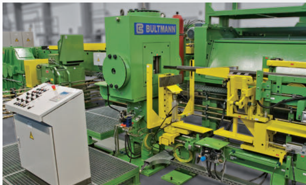
Folding tag pointer HAM 150 for steel tubes, with gripper feed to ensure a continuous production of different point lengths 适用于钢管的折叠压尖机HAM 150，再配以夹持进料，便可确保产品尖端长度不同的情况下，仍能进行不间断生产作业
