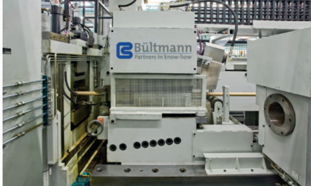
Automatic tube separation, installed upstream of a pointing machine for steel tubes 钢管轧尖机前部的自动管材分放设备
