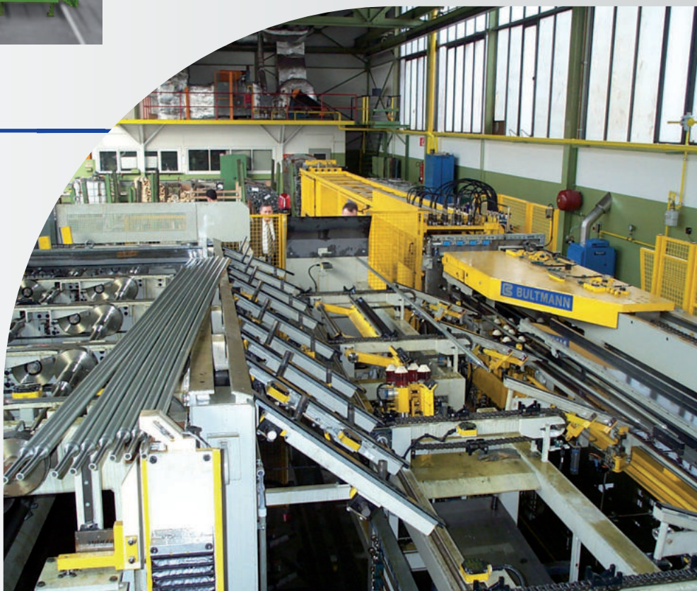
Production line for aluminium tubes with automatic tube separation, with two drawing machines for aluminium tubes, each one designed for 2 x 2 drawing passes, hydraulic shears, testing and sawing units
