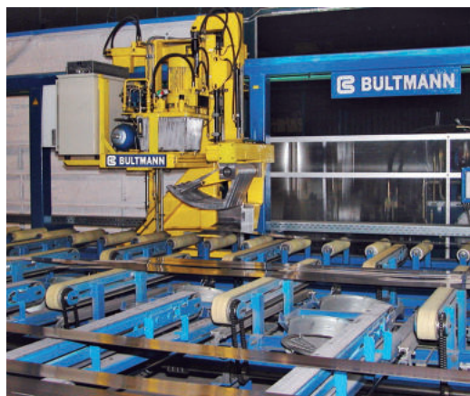
Puller within the runout of an extrusion press for aluminium tubes and profiles 置于铝管材铝型材挤压机出料部位内的拉出装置
