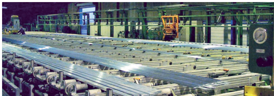
Runout system for aluminium tubes and profiles 铝管材铝型材出料系统
