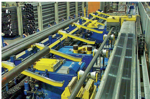
Single tube drawing line for steel tubes, driven by toothed rack, with sawing unit
