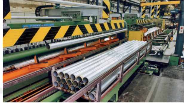
Vacuum transport system for aluminium tubes 铝管材真空运输系统
