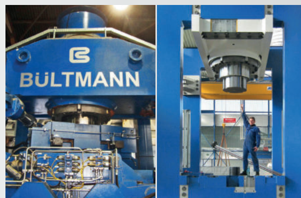
2-roll straightening machine for seamless steel tubes and bars 用于无缝钢管和棒材的2辊矫直机
