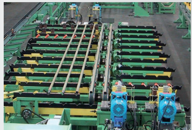
Double chamfering unit for steel tubes, working in line with drawing, straightening, sawing and testing equipment 与拉拔机、矫直机、锯切设备和测试设备协同运行的钢管双倒棱装置
