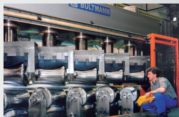
10-roll straightening machine for large-diameter aluminium tubes 用于大直径铝管的10辊矫直机
