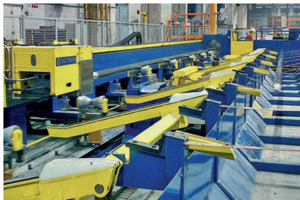
Production line for precision steel tubes, with sawing unit
