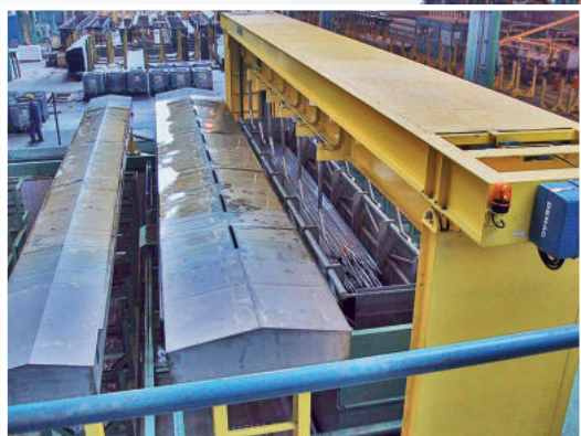
Automatic bundle greasing line for steel tubes 钢管自动成捆润滑加工线
