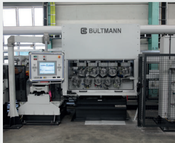
10-roll straightening machine for copper tubes and bars 用于铜管和棒材的10辊矫直机
