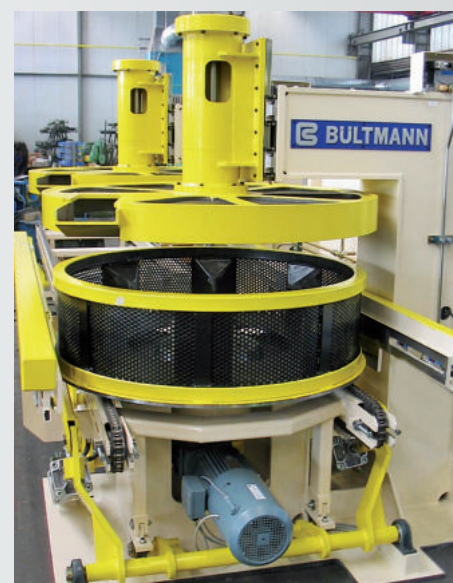
Coiler for copper alloy tubes and profiles, arranged in the runout of an extrusion press 置于挤压机出料部位的铜合金管材型材卷取机
