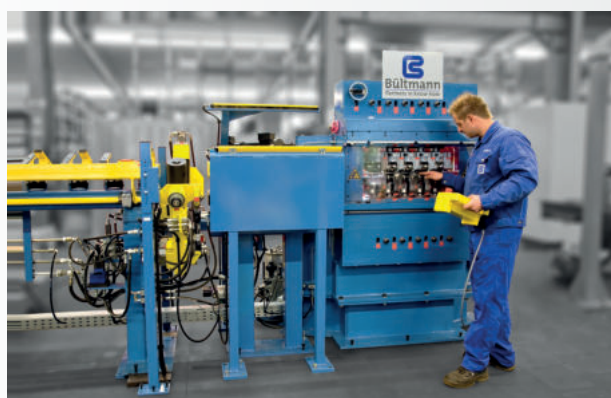
10-roll straightening machine for special steel tubes 用于特殊钢管的10辊矫直机
