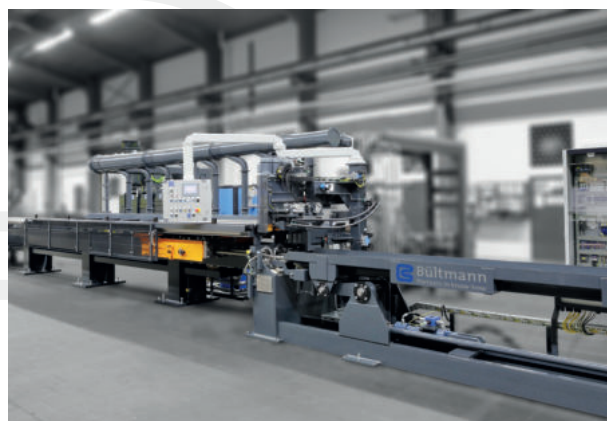
Double tube drawing line for stainless steel tubes, driven by drawing chain
